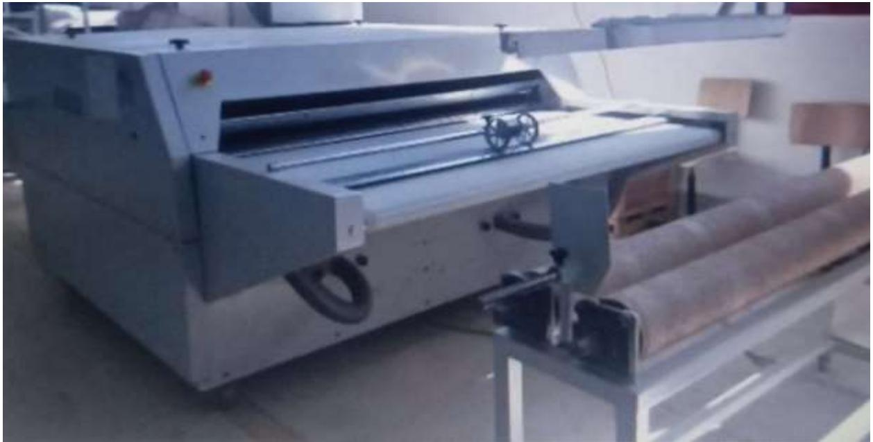
1-rasm. Gazlama sifatini tekshiradigan va nuqsonini aniqlaydigan K 1600 MM markali maxsus dastgoh.
