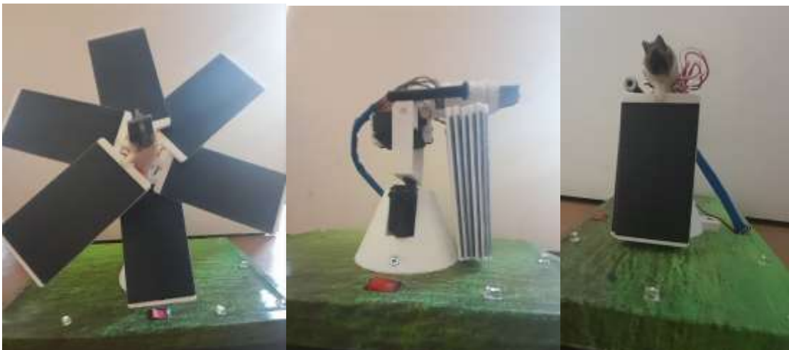
2-rasm. Kungaboqar usulidagi quyosh panellari modeli
