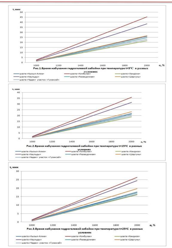
From the above table and graphs it is clear that, at high temperatures and low water hardness, stopes made from hydrogel quickly reach the finished state.
